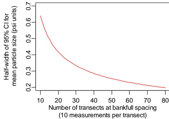
Figure 3. Relationship between number of transects at bankfull width spacing and sampling precision for an estimate of the mean of the sediment size distribution.
