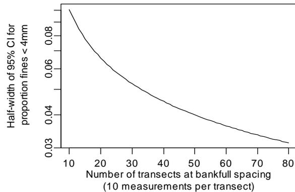
Figure 4. Relationship between number of transects at bankfull width spacing and sampling precision for an estimate of the proportion of the sediment size distribution finer than 4 mm.
