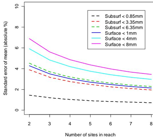
Figure 7. Relationship between number of monitoring sites per monitoring reach and sampling precision for an estimate of the mean percentage of cumulative sediment size distributions less than particular diameters of interest for both surface and subsurface sediment size distributions.
