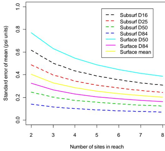
Figure 6. Relationship between number of monitoring sites per monitoring reach and sampling precision for an estimate of the mean of various percentiles and the mean of the sediment size distribution.
