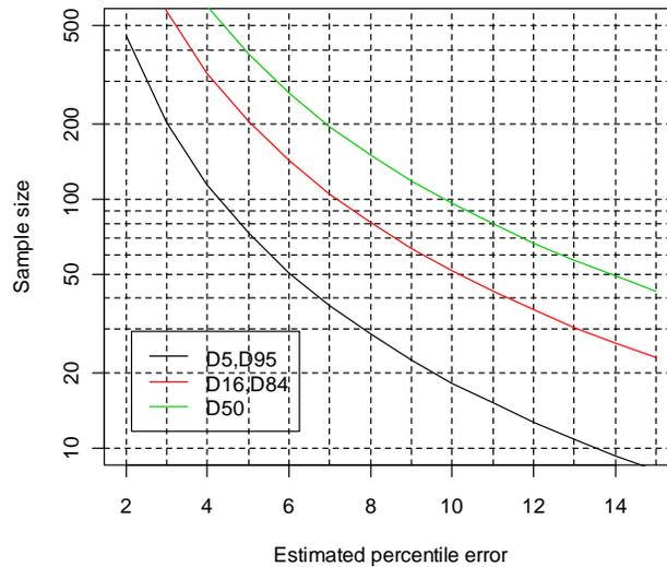
Figure 5. Estimated percentile error for specified percentiles of the cumulative sediment size distribution after Bunte and Abt (2001).
