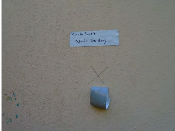
Photo 4-37 ASTM D 3359 / Passed
