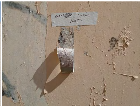
Photo 4-37 Tub ring ASTM D 3359 / result failed
