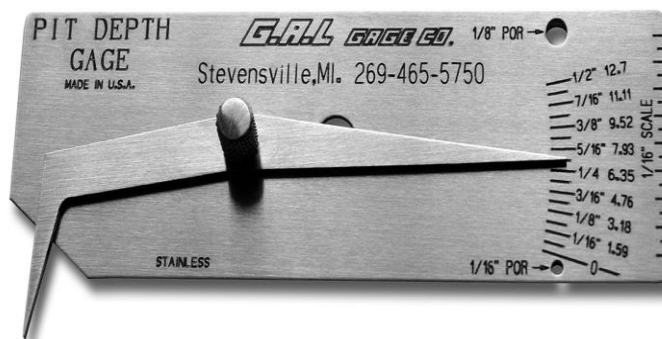
Photo 3-1. Standard Pit Depth Gauge
