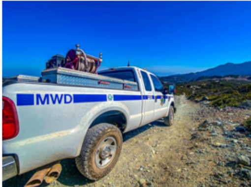
A Ranger patrols the Watershed in a Type 7 Fire Engine. The truck carries a pump and 100 gallons of water.
