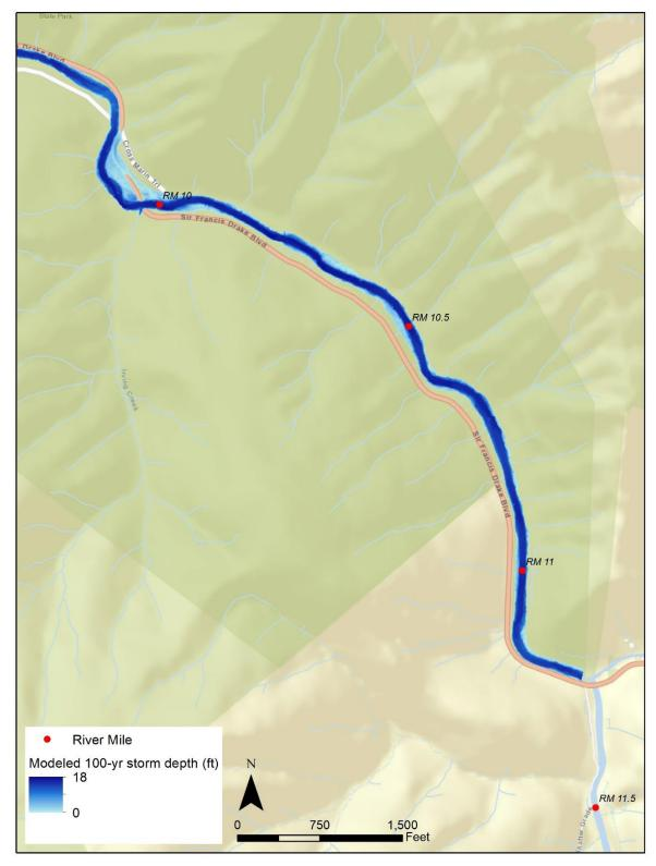
Figure 11b 2D Hydraulic Model Results (Upstream)
