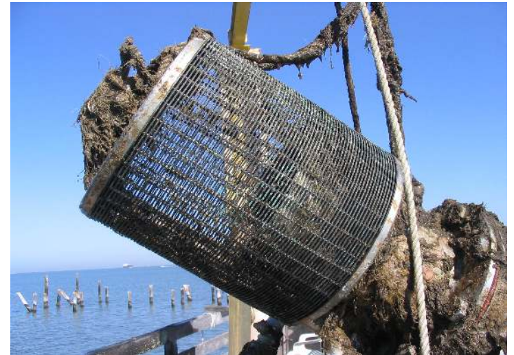
2006 Pilot Facility Intake Screen: 3/32-inch wedge-wire screen
