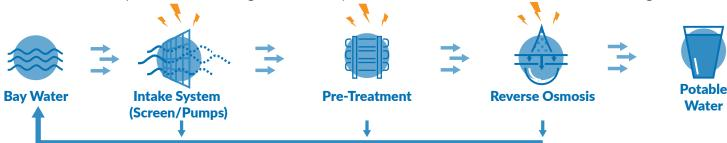
**Temporary** desalination occurs using containerized systems that may be purchased or leased and brought online quickly to address an urgent water shortage. The capacity of each system is limited to what is readily available in the market and could be dismantled at the end of the water shortage.
