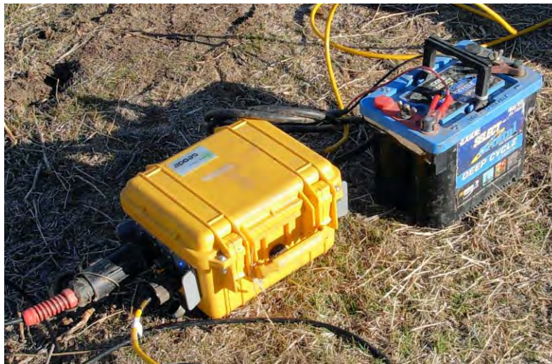
Figure 1: Geometrics Geode 24-channel engineering distributed array seismograph.
