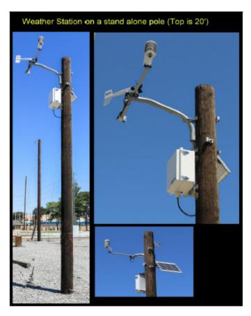
PG&E is deploying approximately 1,300 Weather Stations over the next few years to provide more data around weather during fire seasons to help with possible Public Safety Power Shutoffs.
