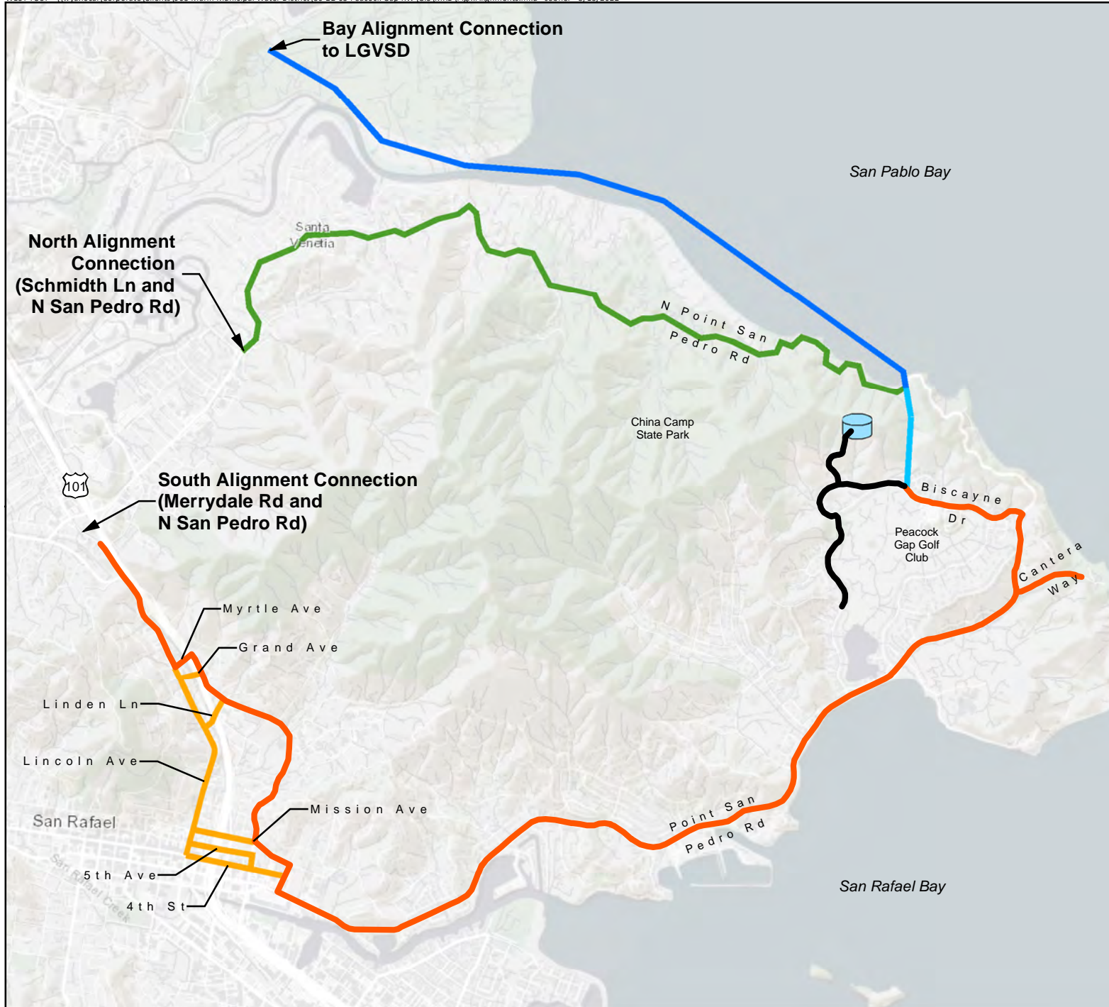
Figure 1 Peacock Gap RW Pipeline Alignment Overview Marin Municipal Water District Peacock Gap Recycled Water (RW) Project
