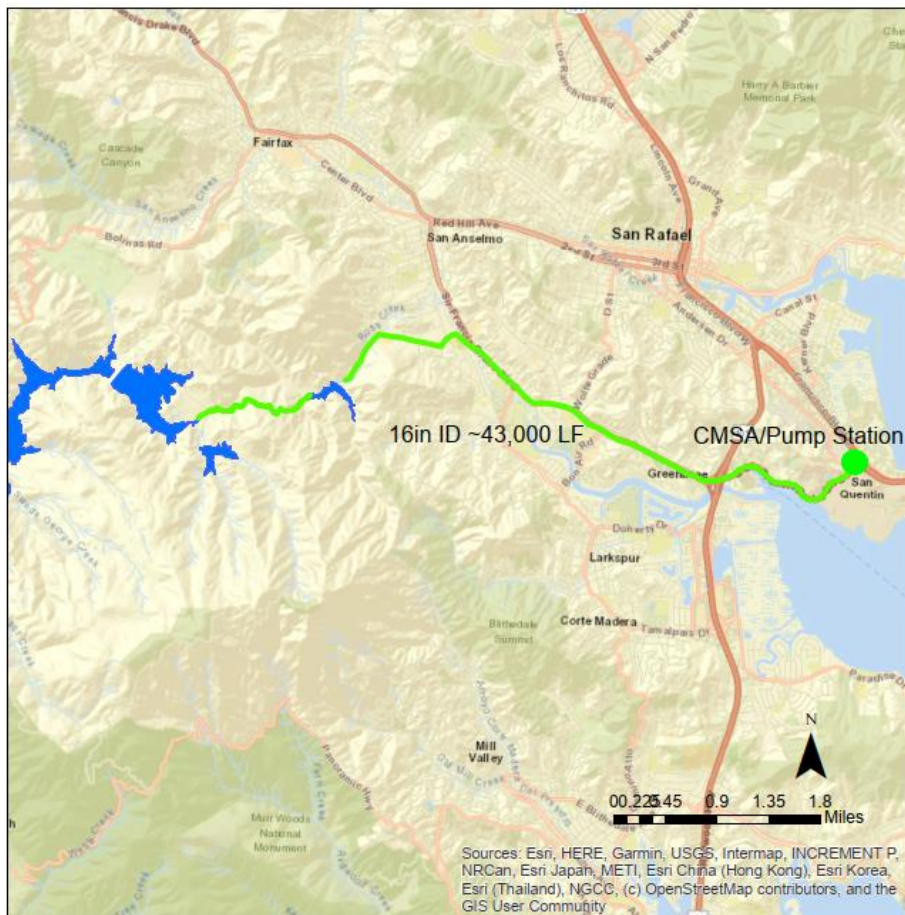
Figure D-23. DPR purified water conveyance concept map
