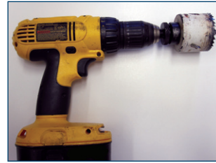
Figure 8. Drill and 2 3/8-inch hole saw.
