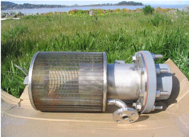
Wedge-wire intake strainer to protect fish and remove large debris (screen dimensions 12-inch diameter by 12 inches long)
