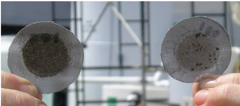
CCM test screens on Bollfilter and Arkal Strainer effluent (Arkal on the right)
