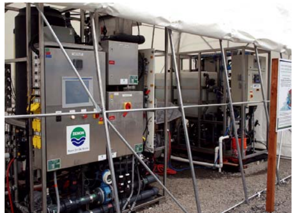
State-of-the-art UF and MF pilot units
